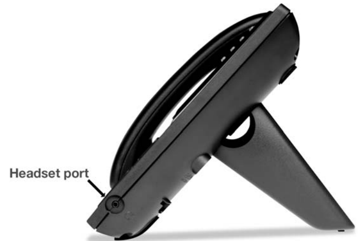
Figure 2-2: desk stand attached to phone (step 5)
